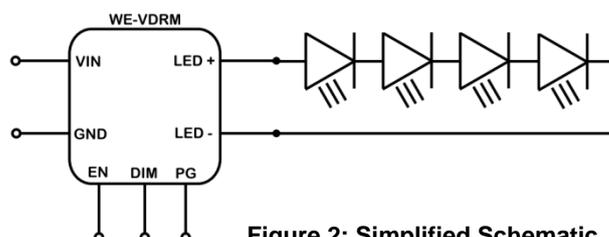
Figure 2: Simplified Schematic
